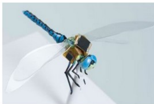
The Draper DragonflyEYE project aims to put tiny 'backpacks' on real dragonflies. Credit: Draper
